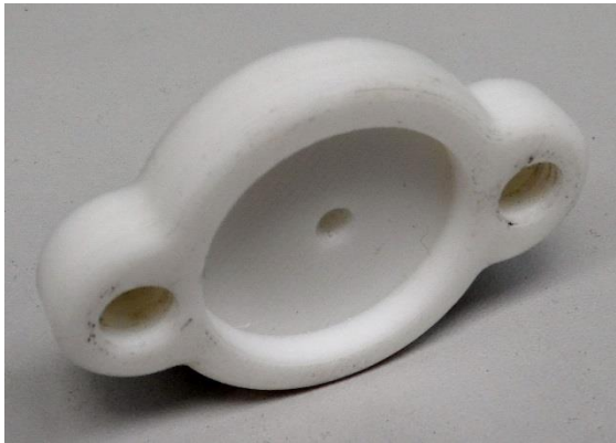
3D Printed Main Piece of the Temperature gauge
